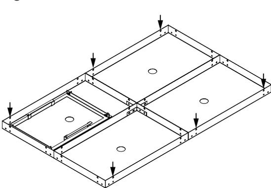
**It is important to pre-assemble the multi pan ceiling before beginning the ceiling pan installation.**
